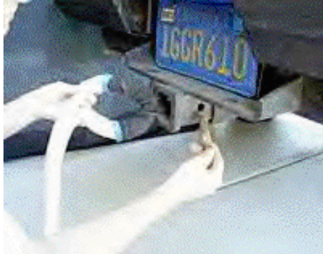
Insert Towline eye into class III trailer hitch and pin.
