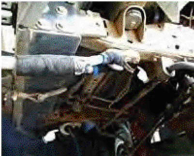
Hooks bolted to frame with hose-protected Towline taped in place.
