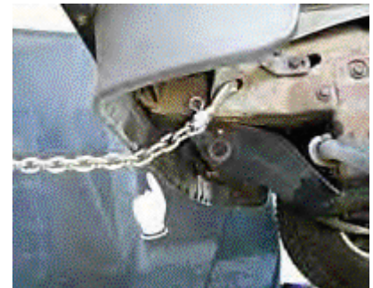
Choke hook in vertical D-hole, but note potential air dam damage.
