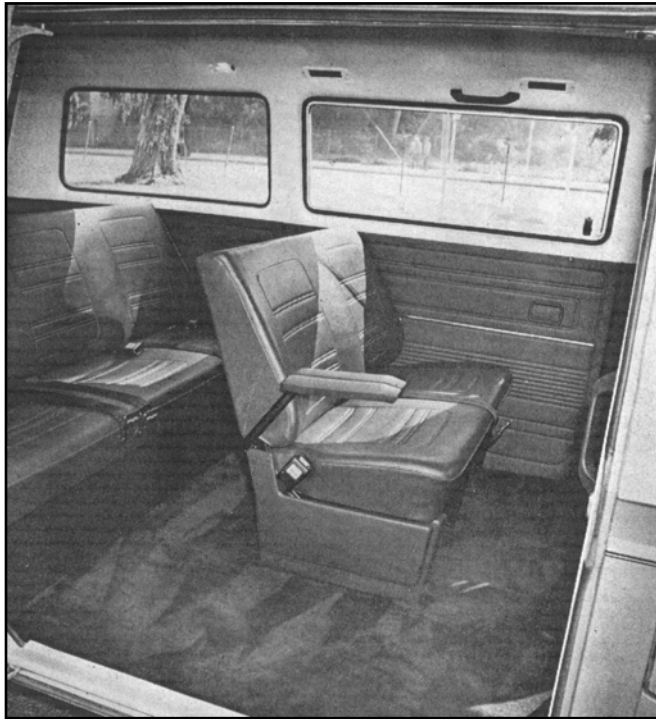
Rear passenger seats show improved design. The side windows are huge and slide open for open-air cruising. Note vent outlets above the window.
