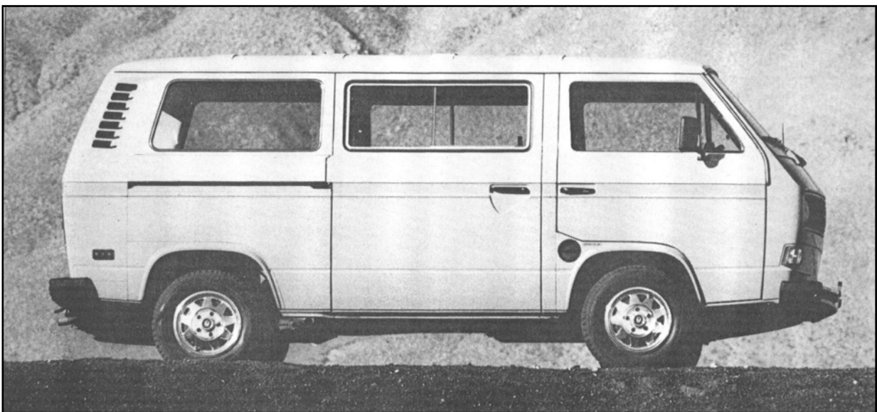
The new sloping windshield is larger than before, but better aerodynamics prevents increased drag. The lowering of the floor creates easier access for passengers through sliding side door. Gas filler underscores new position for gas tank up front for better weight distribution.
